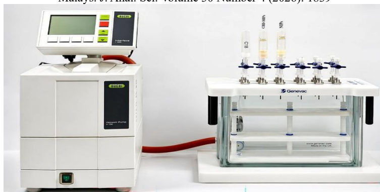
Figure 1. Experimental setup for the solid-phase extraction of cannabidiol using CBD-MIPs
