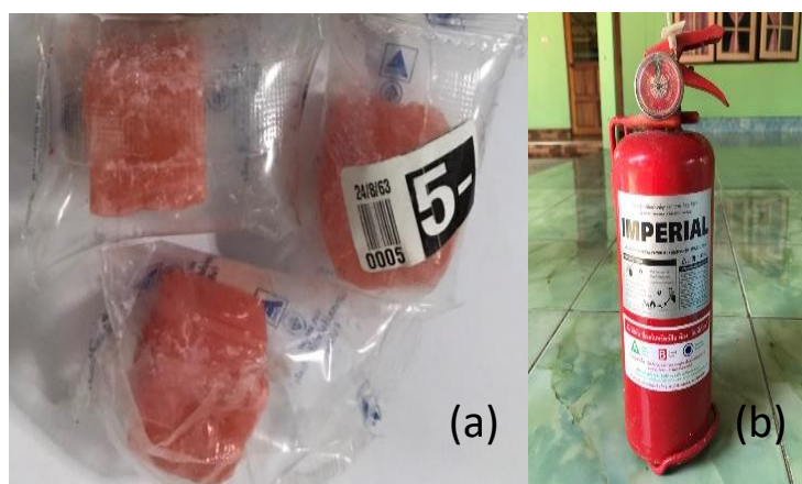
Figure 1. Experimental materials: (a) SAF samples obtained in pink cubic blocks (Brand: RIKO) and (b) dry chemical fire extinguisher employed for suppression experiments (Brand: Imperial, Model: Dry 2.2 lbs)
