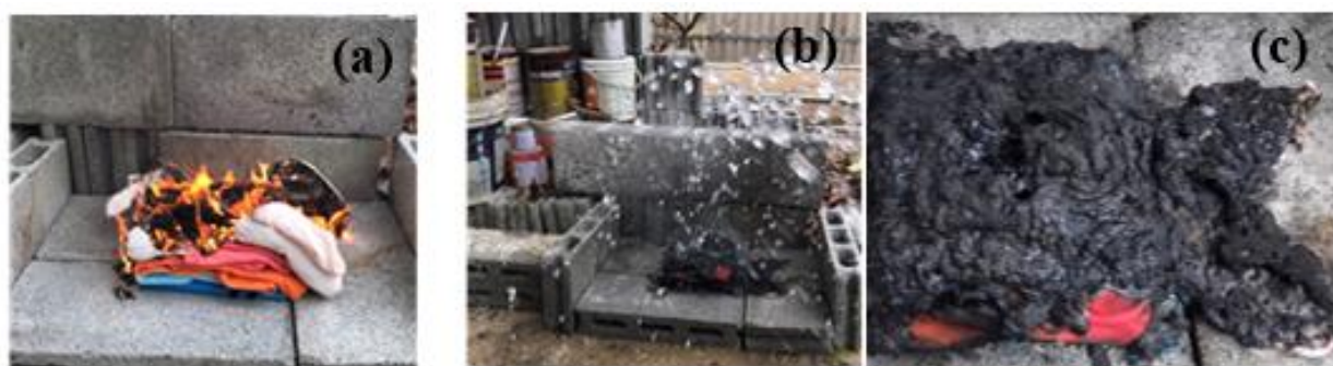
Figure 2. Sampling procedure for charred debris collection: (a) cotton fabric ignited with a SAF block, (b) fire extinguished with distilled water, and (c) a 1 \times 1 \text{ cm}^2 debris sample collected from the central region corresponding to the original fuel placement
