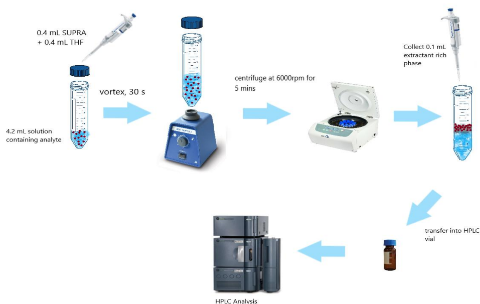
Figure 2. Schematic diagram for SM-DLLME procedure.
