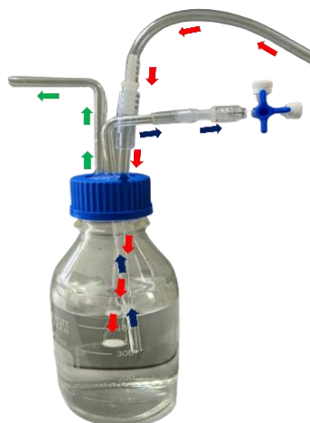
Figure 2. The designed culture flasks in this study. The red and green arrows indicate the air inlet and outlet respectively, while the blue arrow represents the sampling port outlet.
