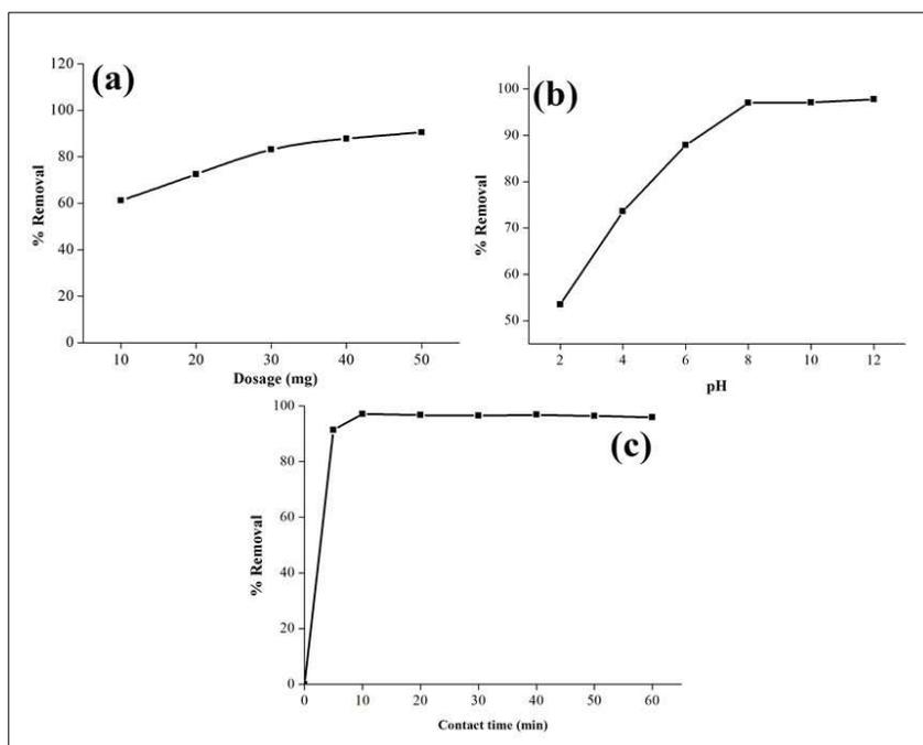
Figure 5. The effect of (a) dosage, (b) pH, and (c) contact time on the sorption of MB
