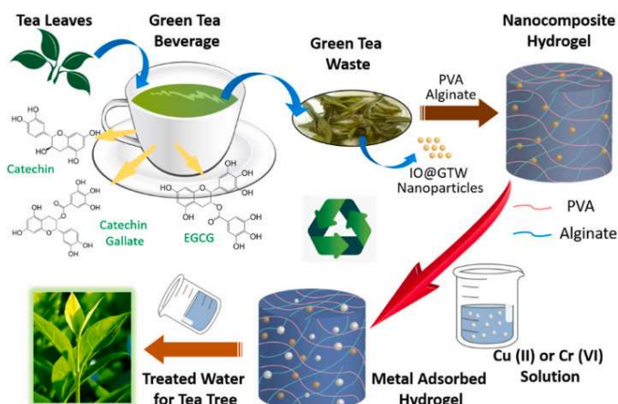
Figure 5. Synthesis of iron oxide nanoparticles by using green tea waste. Iron oxide nanoparticles were blended into PVA-alginate hydrogel to form PVA-alginate- \text{Fe}_2\text{O}_3 nanoparticles as a binder of \text{Cu}^{2+} and \text{Cr}^{6+} in an aqueous solution. The treated water was re-used for tea cultivation [31]
