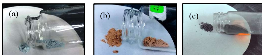
Figure 1. (a) Undoped \text{SnO}_2 , (b) Co doped \text{SnO}_2 , and (c) Pd doped \text{SnO}_2 powder samples
