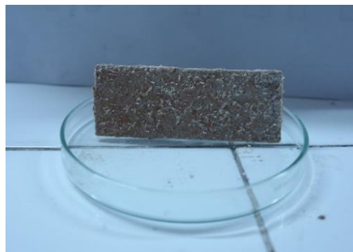
Figure 3. Deposited matter at cathode
